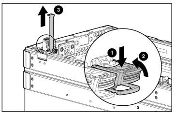
Figure 1-25: Removing expansion board blanks
